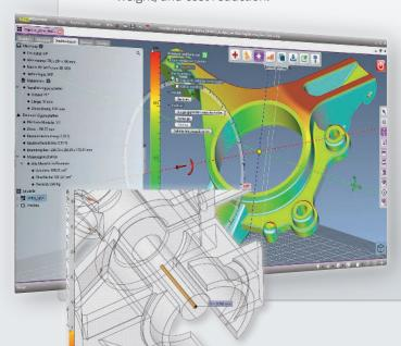
The orientation analysis tool includes up-and-down skin detection, geometric roughness, and support accessibility. Up-and-down skin works perfectly in combination with our SLS and SLM Buildmanager. The roughness analysis function allows the user to analyze the stair-stepping effect in relation to the orientation of the part, before printing. The supports accessibility identifies the potential complexity for removing supports.
