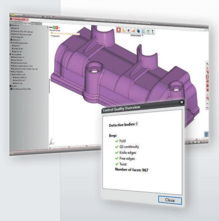
Superior manufacturing quality is guaranteed by the hybrid geometry kernel that handles STL files but also exact and light CAD geometry, in accordance with the VDA 4755/2 engineering standards. Interfaces for 24 major formats like CATIA, NX, SOLIDWORKS, Creo, STEP, and JT also provide 3D dimensions and tolerances, views, attributes as well as CAD design features.
