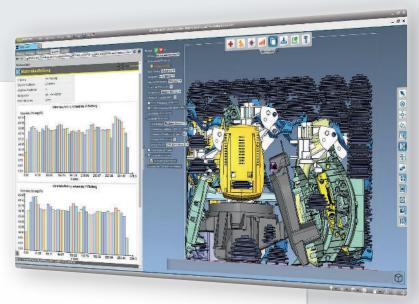
For mass production, the new power copy function allows for extremely fast packing of identical parts with maximum packing density. A report is generated, showing the even distribution of the nested parts.
